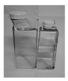
Remove aluminium foil from the air connectors of both vessels and attach the air filters via the silicone tube. IMPORTANT: Avoid touching the connectors and edge of the silicone tube with your hands. Once air filters are attached, remove the aluminium foil from the media connectors and attach the media transfer silicone tube. After this step, the bioreactor is successfully assembled.
