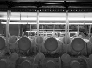
SETIS™ bioreactors are designed to be placed side by side, and back to back, without losing any shelf space, with the advantage of having all connectors and caps at the outside of the shelf.
