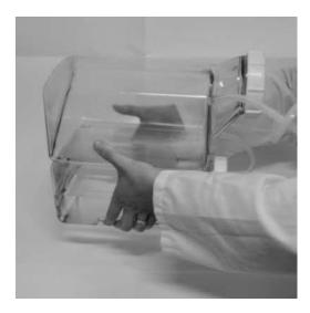
Place the bioreactors on a perfectly horizontal and hard shelf surface. The bioreactor has the required inclination to allow self-drainage following the immersion phase. This inclination can be altered by irregular and/or wavy shelf-surfaces, compromising a correct media drain.
