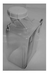
Silicone gaskets are designed to fit tight into the inner side of each cap, to prevent the silicone gasket getting loose from the cap, once the vessel is opened under sterile conditions. Place the silicone gasket into the cap and screw it onto its corresponding vessel. The edge of the vessel's neck will push the silicone gasket uniformly into its place.
