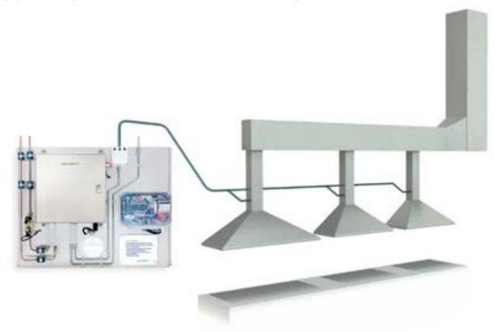
A single RENA system can treat both small and large air flows in the kitchen ventilation - up to 12,000 L/s  $(43,000 \text{ m}^3/\text{h})$  at medium grease load.
