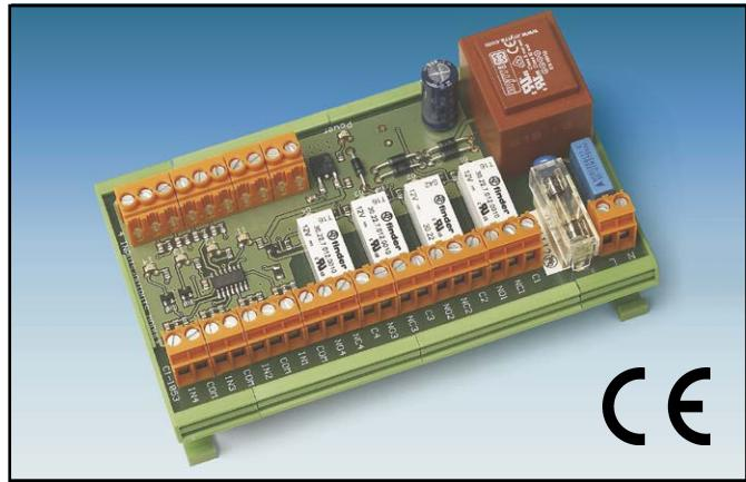
This module is a conversion unit that directly connects the logical inputs and outputs of the SMART indicator and provides the user with 4 contact inputs and 4 relay outputs as well as the necessary power supply.
