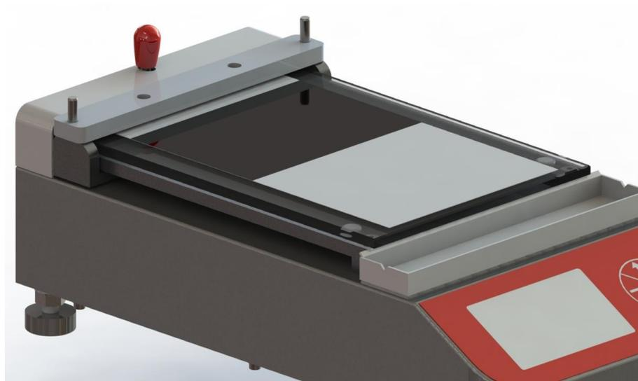
Place the quadrangular applicator in the centre, touching the slide bar
