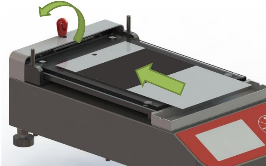
Once it is properly positioned, release the lever so that the contrast card is secured.
