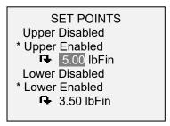
Either one, two, or none of the set points may be enabled. To toggle between the clockwise and counter-clockwise directions, press the **DIRECTION** key.
