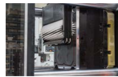
Brush and demoulding systems Fully automatic demoulding devices and brushes for production of precise O-rings, seal elements and mould articles
