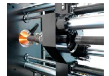
FIFO Duale On request, various MAPLAN FIFO injection units are available with hydraulic nozzle lift-off for flexible adaptation to different tool situations
