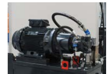
Hydraulic drive Reliable hydraulic drives with axial piston pump design
