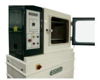
√ 8 round bars specimens support of 12 mm of material nonmetallic.
