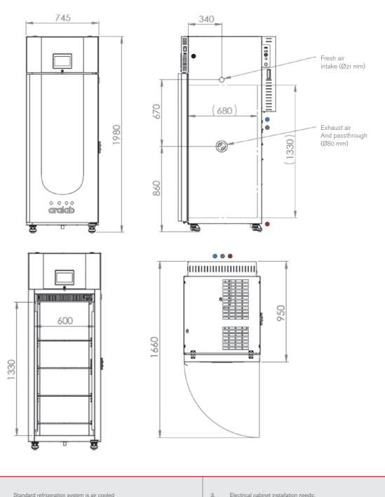
Standard refrigeration system is air cooled 1.
