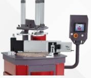
The AUTOPLAN system enables effective management of plate flatness and grooving. It is positioned and dismounted in a few minutes thanks to the dedicated fixation points integrated in the machine.
