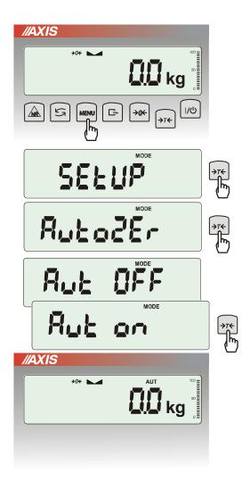
When the function is activated, the scale automatically ensures stable zero indication if the pan is empty or if zero indication was acquired by pressing  $\rightarrow T \leftarrow$  key.
