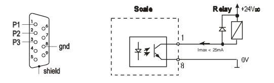
*Relays* output is the open collector transoptor output with load capacity 25mA / 24V. Transmitter inputs must be protected with diodes, e.g. 1N4148.
