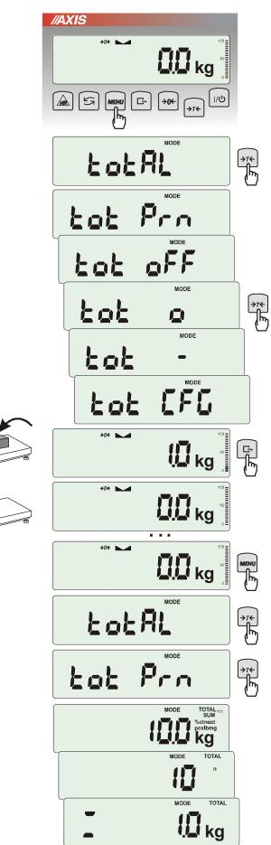
The function allows calculating total weight for series of measurements, which can be greater than scale capacity. It allows calculating total weight as well as average value.
