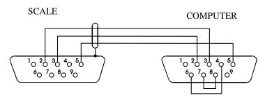
Connection cable WD-1 (connects scale with AXIS printer):
