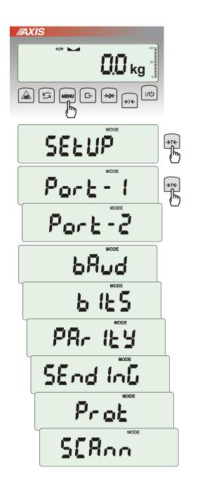
17.4 Serial port parameters setting (SErIAL)
