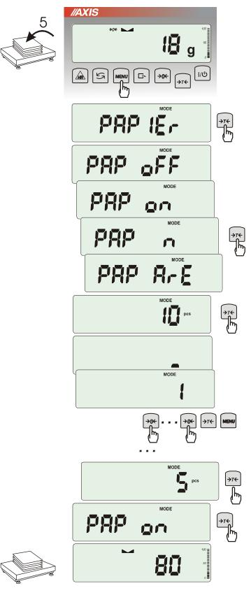
This function enables to calculate paperweight of  $1m^2$  of paper basing on samples of known area. For quick access, the function is accessible directly by pressing *MENU* key.
