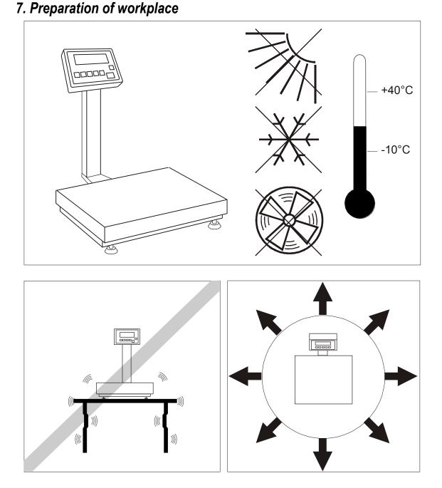
The workplace should be carefully chosen in order to keep to minimum influence of external factors that can disturb balance work. Proper temperature and work space is crucial. Balance should stand on stable foundation made of non-magnetic impact material.
