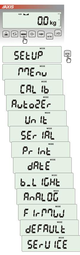
*SEtUP* contains all options used for setting scale work mode:
