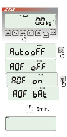
The function is helpful in scales supplied from accumulators. The function causes scale to switch off automatically.
