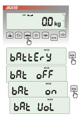
*bAttErY* function allows switching on or off charging accumulators during work with feeder and checking their power level.
