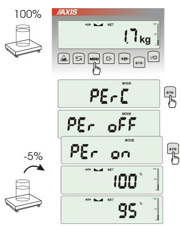
This function allows displaying weighing result in percents.
