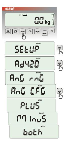
This option enables to set-up analog out (4-20mA or 0-10V) working method used e.g. in PLC regulators:
